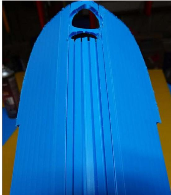
NOTICE that the holes for the dowels are not made yet. This is done by carefully folding the fuselage around the pine formers and piercing through the plastic with an awl or screwdriver. This requires a strong grip but it's possible to adjust and twist the plastic edges so that they align accurately with the lower edge of the wood former. The pre-drilled hole in the wood guides the screwdriver.
