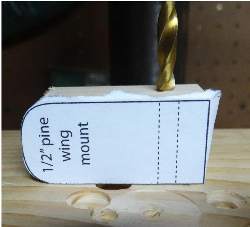
I used 3/16" wood dowel that I bought at Lowe's for the "pins" that hold this plane together. It is IMPORTANT to know that the pins will not be glued into the wood mounts. They need to be moveable for assembly. Drill the dowel holes for a sliding fit but size and position don't need to be critical. The following picture shows the groove for the landing gear cut into the forward face of the engine mount.
