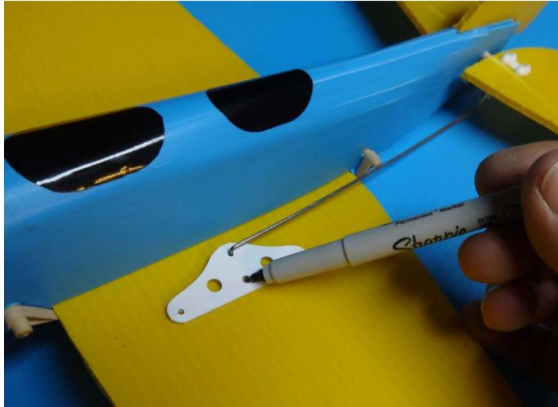
Here are the finished controls. Notice that the bell crank is on top of a stack of plastic washers about 3/8" high. The pivot bolt is a #4-40 with a "Nylock" nut.
