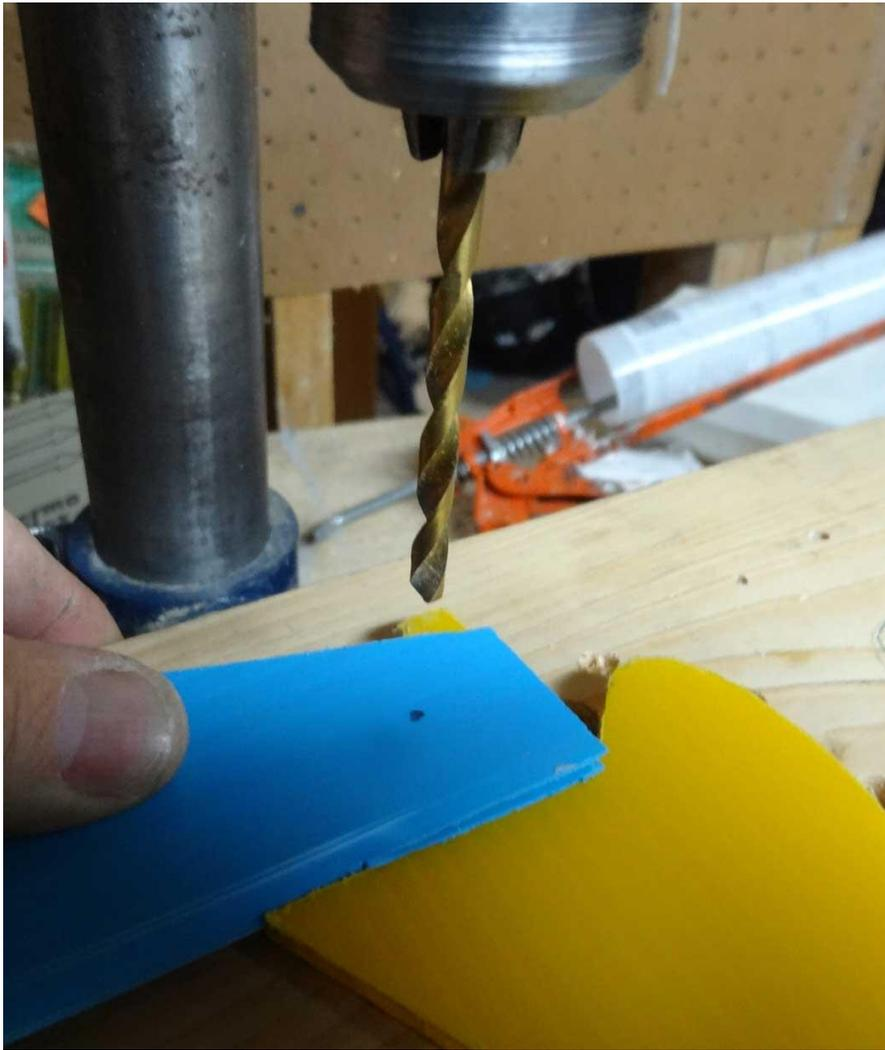
A nice clean hole! A 3/16" Forstner bit works well, but a regular, and sharp, drill bit works OK if you cut slowly.
