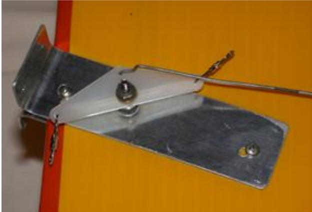
The bellcrank is a standard  $\frac{1}{2}$  A type (either metal or nylon would be OK) which you can purchase from most hobby stores, along with a suitable small control horn. You then connect the bellcrank to the horn via a pushrod made of .049 piano wire.
