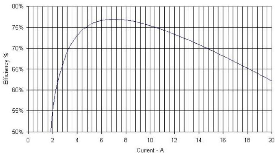
The graph above is for EMAX2822 used in my indoor planes. It shows the max. 77% efficiency when the current is about 7 Amps. EMAX2822 in my Bee1 and Wasp draw 8.2-8.4 Amps. statically and about 6 Amps average in air ( $\frac{3}{4}$  Rule). At 6 Amps the efficiency of EMAX2822 is 76% - not bad.
