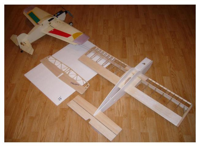
Modified LGW (top left) with Cobra 2814/12 instead of Cobra 2808/22, larger wings (328 sq.in instead of 286 sq.in.), 9x6 APC pusher, 30 Amps. ESC, KR governor, 3S 2200 mAh. 30C battery. Weight RTF: 795 grams. (28 oz.).
