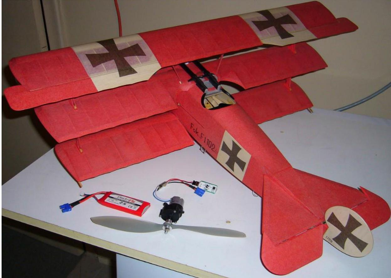
I have flown this model today on 5.5 m. long “SpiderWire” lines, using the 2S LiPo, 370 brushed 6.6:1 geared motor with the 10x4.7 APC slow flight propeller and 12Amps Eflite ESC for brushed electric motors. The timer: Eflite EFLA172.
