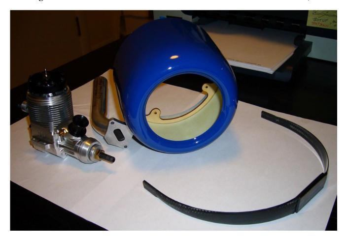
RO-Jett76 with header/muffler will be mounted in the horizontal configuration (the engine cylinder to the outside of the circle).
