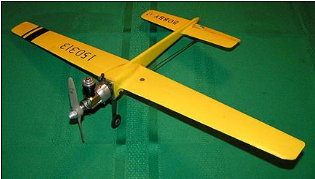
Paul Gibeault's World Record holding Streaker, 2:14 Heat; 4:22 Final This mouse racer features a CNC cut semi-symmetrical wing airfoil, symmetrical flat stab, and removable titanium landing gear. Powered by a Cox Venom, burning 65% nitro and 15% propylene oxide fuel.
