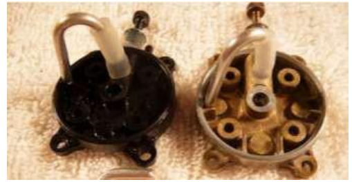
The replacement pick up tube is bent from 3/32" O.D. soft aluminium tubing & chamfered at the bottom to fit exactly. Silicone tubing attaches it to the tank back.
