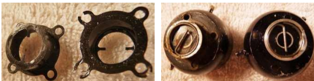
Black Widow tanks: note severe wear around reed flange holes on reed retainer (Left) excessive wear on top of reed retainer (Right) cracked retaining "GClip" area and reed seal venturi hole area.
