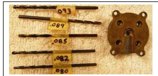
One not fully explored area of performance is tank venturi & tank back mis-match. It is thought preferable (& sometimes works) to have the tank backplate venturi a few thou. **smaller** than the tank venturi. A too large tank venturi (i.e. .089") can sometimes be made to work with a smaller .082" tank back.
