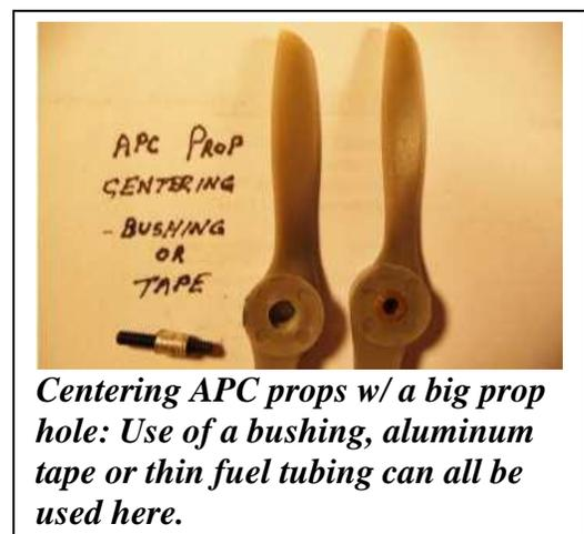
*Centering APC props w/ a big prop hole: Use of a bushing, aluminum tape or thin fuel tubing can all be used here.*
