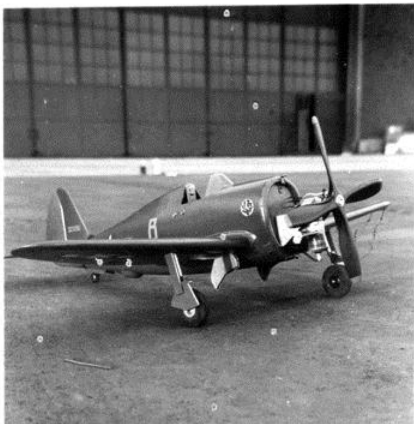
A joint build between Clarke and Ralph Bolitsky of Guelph. Picture was taken at RCAF Debert, Nova Scotia in June of 1945. It has a hand carved wood prop. Clarke carved nearly all of his props himself. Note the control wires hanging from the port wing.
