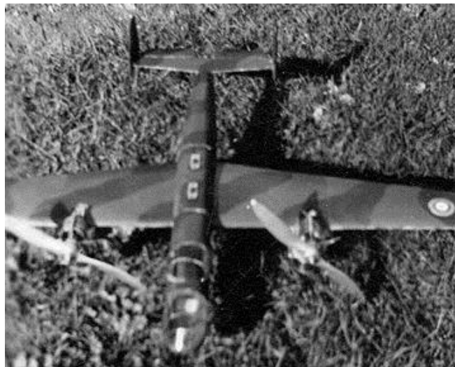
Clarke's scratch-built B-25 Mitchell control line model with twin Forster .29's was all carved from solid balsa! It had a 30 inch wingspan, approximately. Picture taken in Toronto in 1942. You can make out the twin switches atop the fuselage for the ignition.
